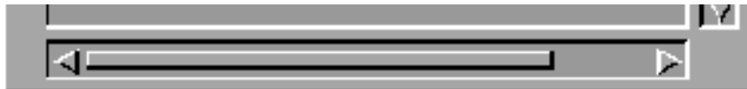
Figure 1-2 A QPANEL item with an ACTION,HS attribute to create a scroll bar
