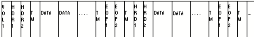
Figure 5-1 Vault Tape Format
