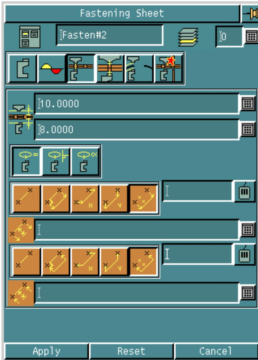
2. Specify a value for the ride height for the upper anvil in the Upper Ride Offset field. This is the distance the lower anvil moves to before positioning to each point in a fastening feature.
