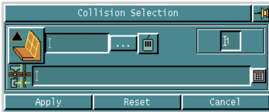
2. Click the list button. Choose a collision surface feature from the Features scroll list that appears and click **Accept**. The selected feature appears in the Collision Surface field of the Collision Selection sheet.
