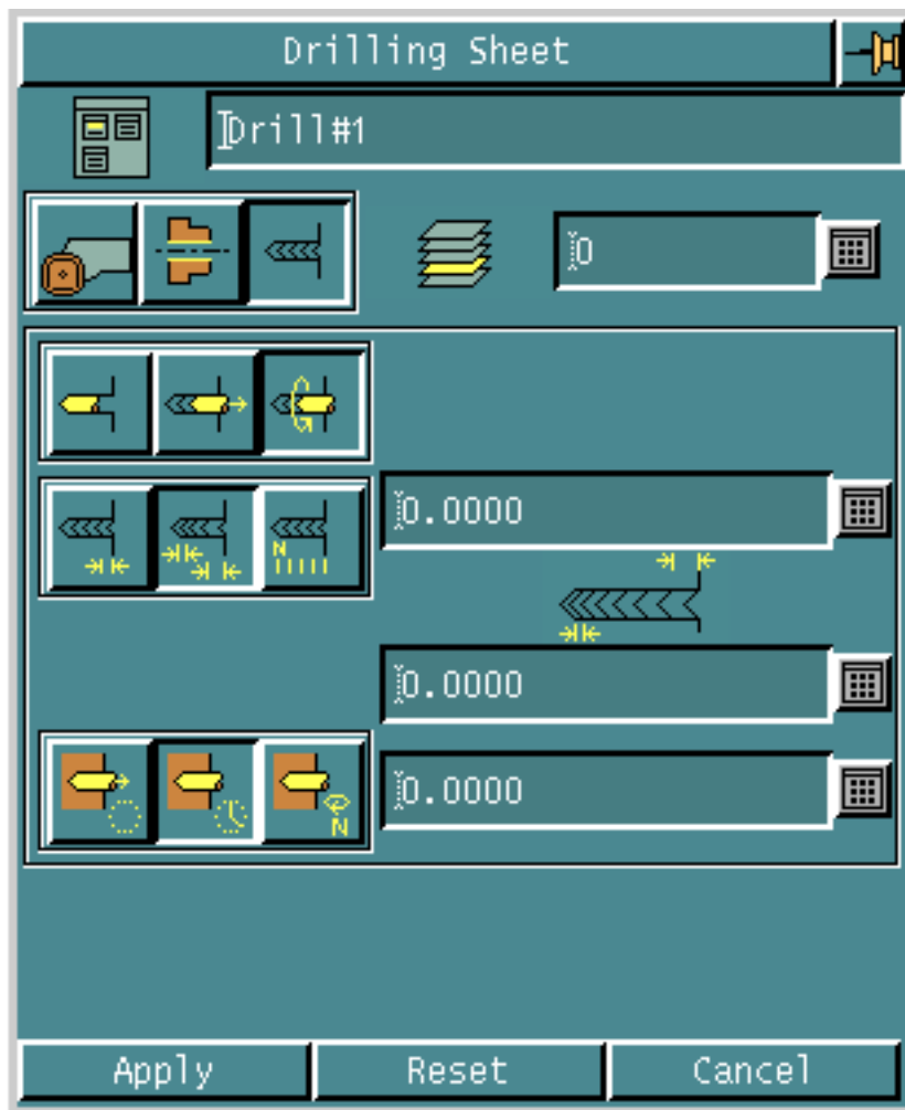
Figure 7-8 Drilling Sheet for General Parameters
