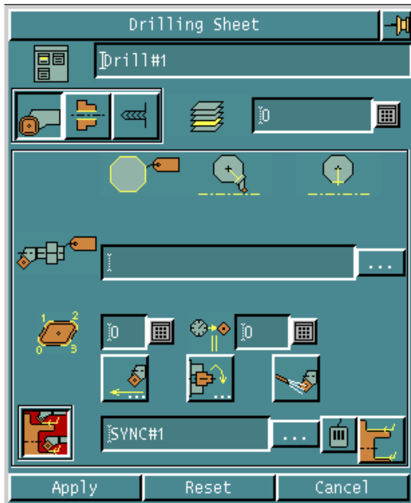
Figure 7-3 Drilling Sheet for Tool Assembly Selection Parameters
