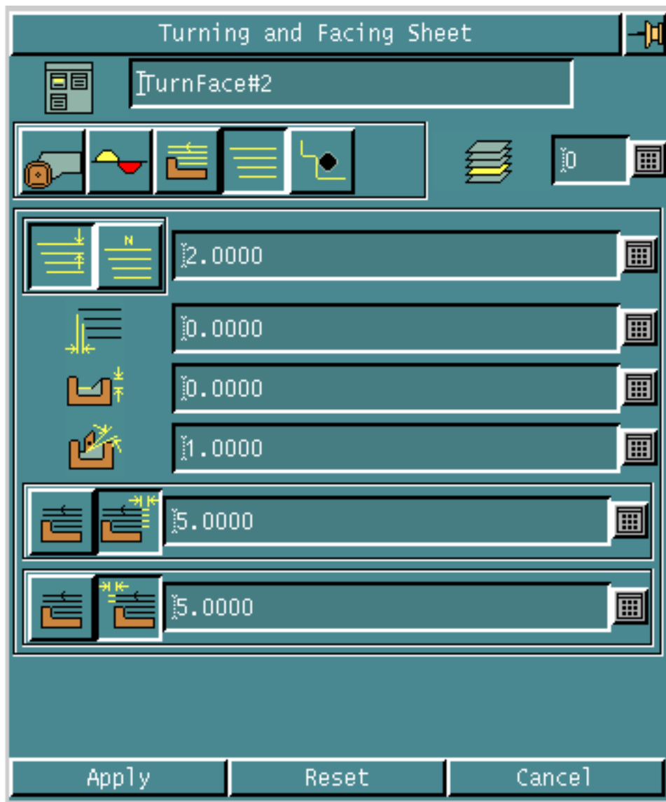
Figure 5-18 Turning and Facing Sheet for General Parameters
