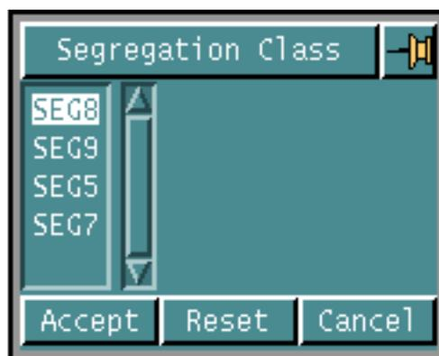
Segregation classes are used to determine which wires can or cannot be routed along a channel segment. Specifying a segregation class on a channel segment affects the automatic routing of wires. Wire segregation classes are defined in the netlist file. Only wires with a matching segregation class can be routed along a channel with the same segregation class. This value is stored as an attribute `segclass` on the channel.
