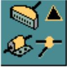
Choose the Edit Harness Component option from the Harness task set to edit the attributes of an existing component in a harness model. Choosing this option displays a property sheet for editing various attributes of the selected harness component.
