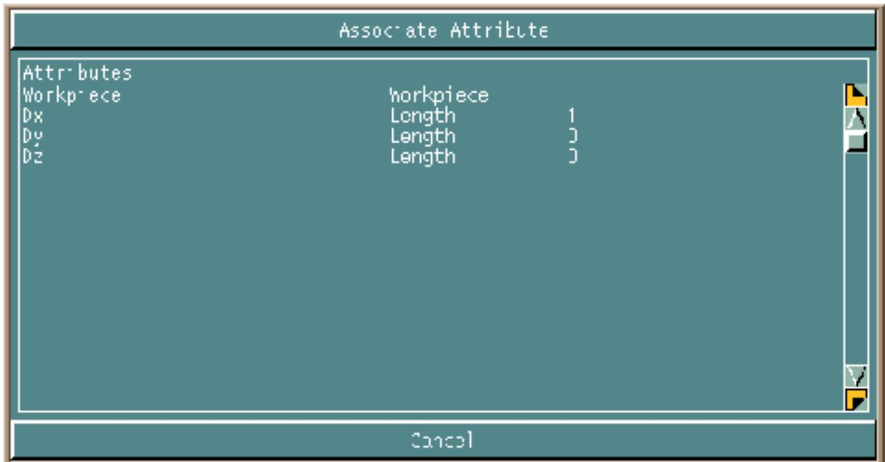
**9.** Click **Workpiece** and then select the connect-point geometry on the screen. Similarly, you can select other attributes from the scroll list and attach them to the new geometry.
