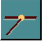
Choose the Insert Junction option from the Insert Components palette to insert a junction into a harness model. Choosing this option displays the Insert Junction property sheet.
