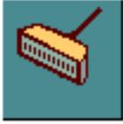
Choose the Insert Connector option from the Insert Components palette to insert a connector into a harness model. Choosing this option displays the Insert Connector property sheet.
