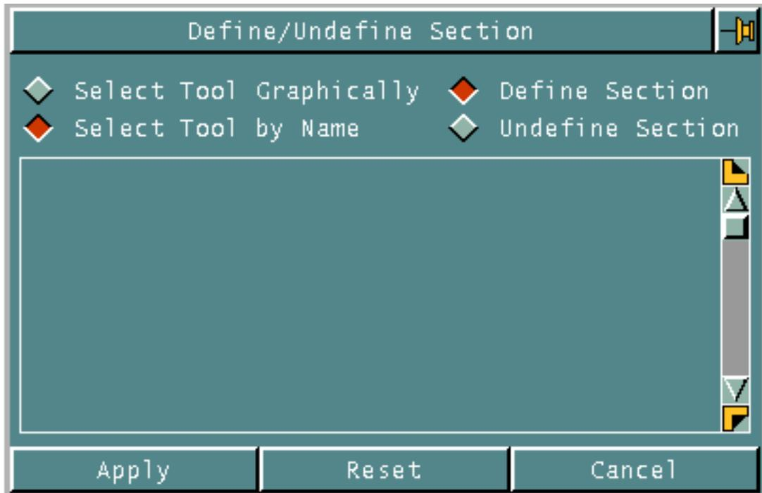
The Define Section option allows you to specify which section cutting tool cuts which solid object in which view.
