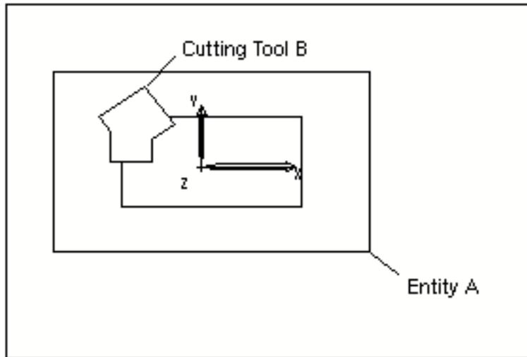
If the relevant section cutting tools do not intersect, create a third section cutting tool and then boolean all the three section cutting tools together.
