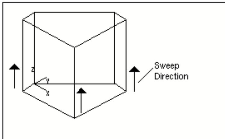
By conducting linear sweeps, you can also produce cutting tools of a more complex shape. An example is given below.
