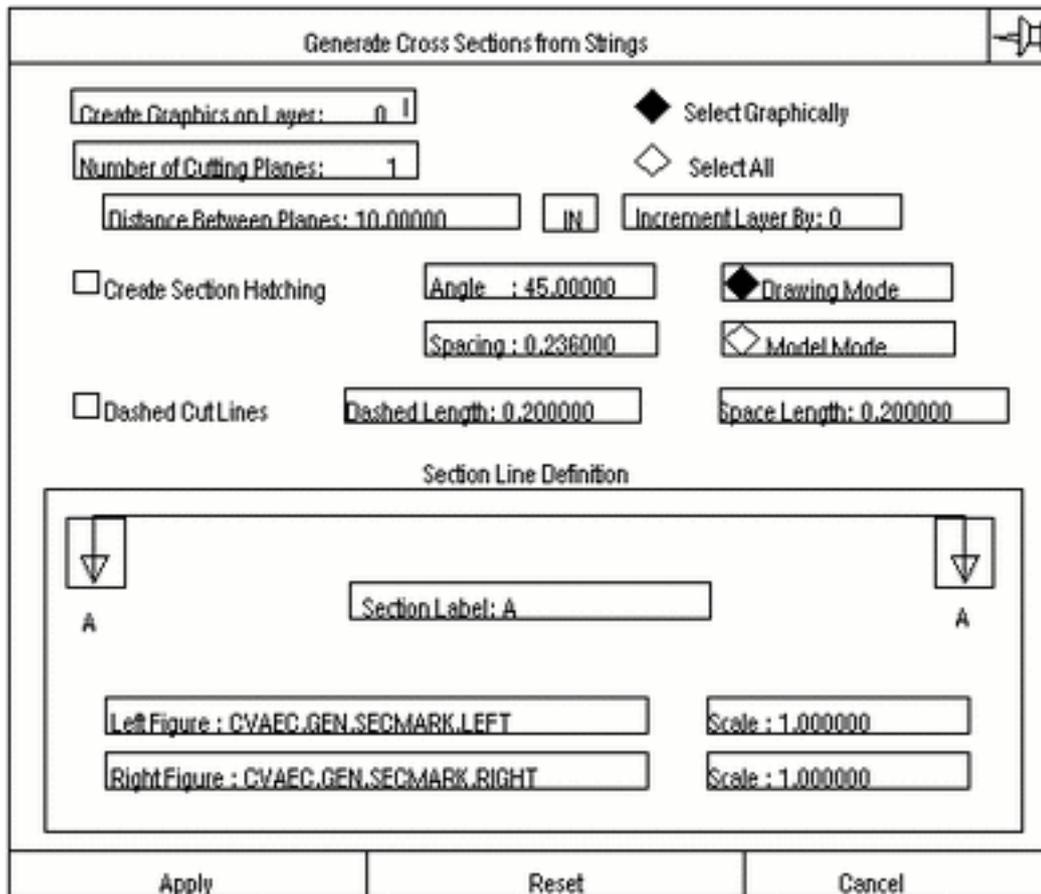
2. Enter the layer number in the Create Graphics on Layer field. The line entities representing the section are placed on this layer. The active layer is the default layer.
