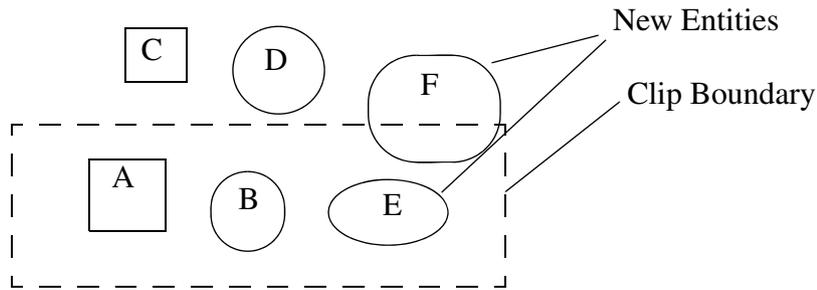
Entities F and E are not in the database for sectioning as they were created after running the sectioning or regenerate command. Now, running the command **REGENERATE SECTION** with various modifiers will show behaviors respectively as follows:
