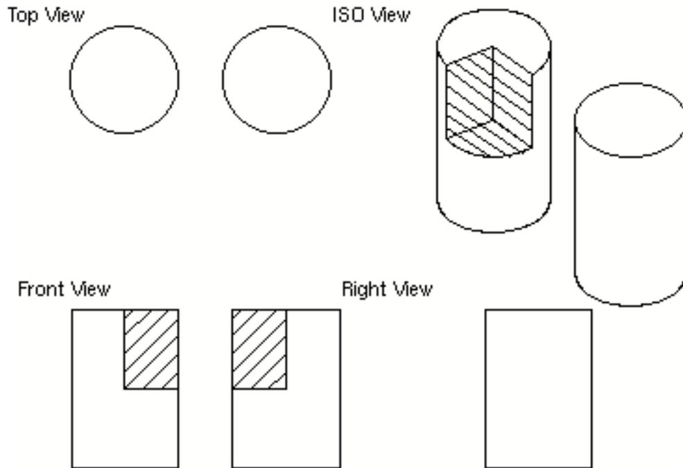
When the isometric view and then the front view are selected, the leftmost cylinder appears sectioned in the isometric view and both cylinders appear sectioned in the front view. The sections are crosshatched.
