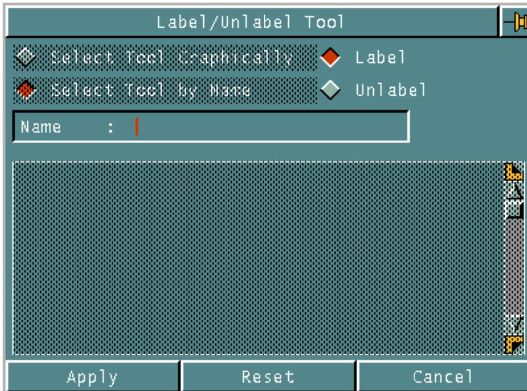
The Label option allows you to identify by name the solid entity that will be used as the section cutting tool. This step is compulsory for any subsequent sectioning operation. An entity can only be used as a section cutting tool in a sectioning operation, if it is first named as such in the database.
