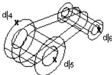
Subtracting the inner cylinders from the outer cylinders
