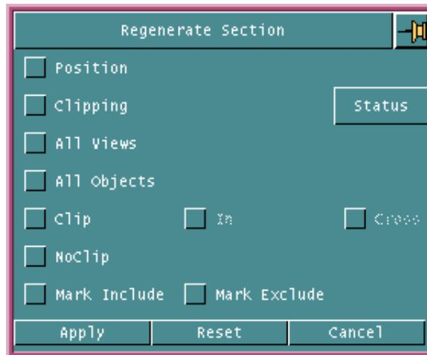
2. Choose Position to align the display view with the alignment direction defined by the Define Section command (shown by arrows on the screen).
