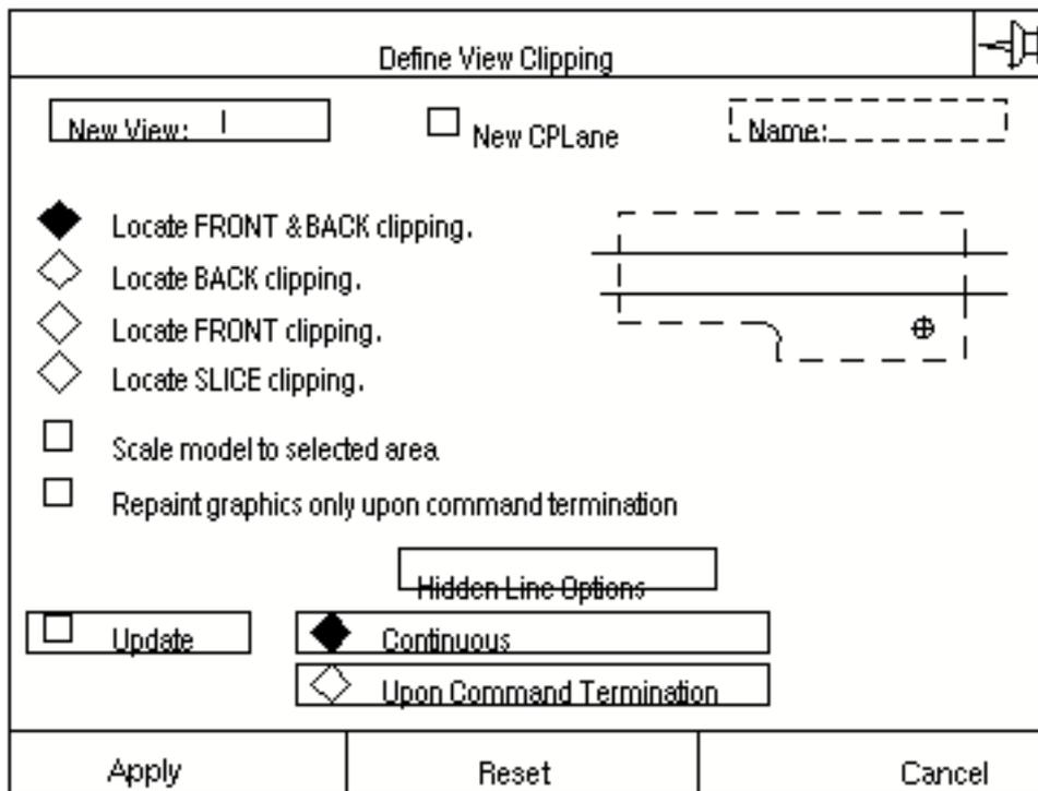
2. Enter a name for the new view being created in the New View field. The name of the view can be of up to 20 characters in length.
