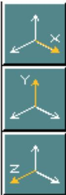
Points the selected axis in the direction of the axis selected on the direction menu (PX, PY, PZ).
