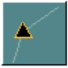
You can add an additional vertex to an existing String or Nline. The new vertex can be used to reshape any String or Nline by replacing any segment with two segments joined at the new vertex.
