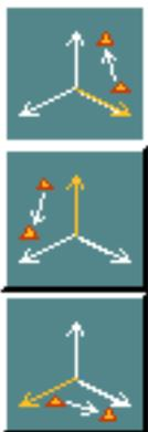
Turns the x-, y-, or z-axis in the direction of a selected line or vector (TX, TY, TZ).
