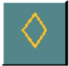
A Cnode describes a coordinate location in space that is used as a predefined attachment point for Nlines, symbols, figures, and text. It is associated with all Nlines and figures you select.
