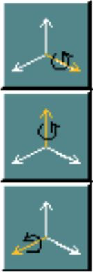
Rotates the instance the given number of degrees about the specified axis. Rotation is clockwise with respect to the positive direction of the axis. By default, they refer to the axis in model space (TOP Cplane). All rotation is done about the origin of the instance. If AX, AY, or AZ are not used, the default is 0 degrees rotation.
