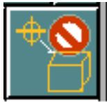
**Deleting Detailed Objects:** This enables you to delete detailed graphics from a model or portion of a model, returning it to its predefined state. If a detailed entity is digitized, the command deletes all Draw View mode detail graphics associated with Nfigure or Nline, and fonts on all strings related to a projected outline.
