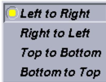
You can specify the position where you want to place the root node and the corresponding child nodes in the assembly tree display, using the options shown in the above window.
